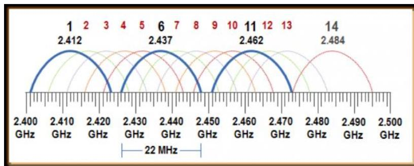
The diagram above depicts a spectrum analyser view of the frequency space occupied by these 14 channels. Within the 2.4 GHz band, only three channels have non-overlapping frequency space: channels 1, 6 and 11.
