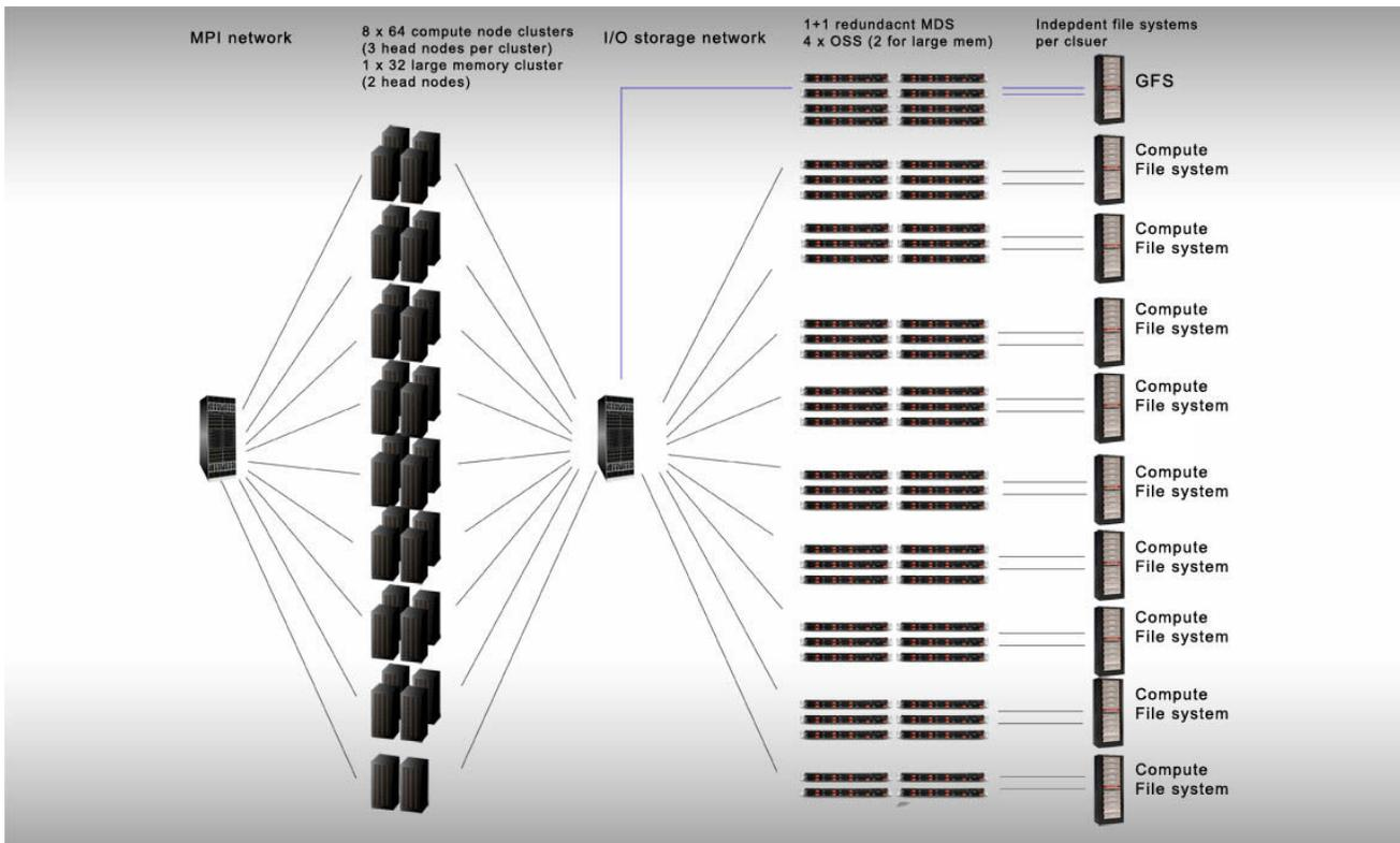
The high-speed interconnect is completely split between I/O and MPI traffic to ensure maximum performance regardless of the job. Both types of traffic use QDR InfiniBand with up to 40 Gb/s of bandwidth, and this interconnect goes directly to the storage controller.
